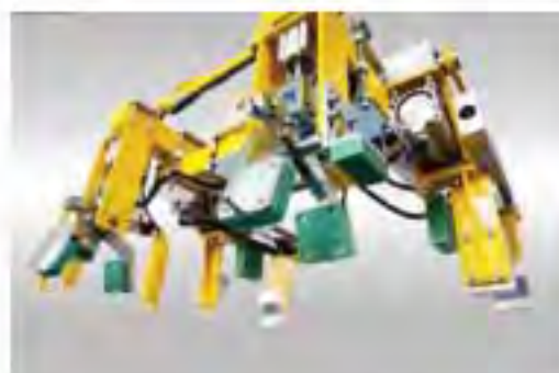
End effector tooling for handling Rear Axles
