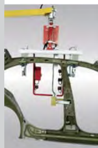
Fixed Overhead Rigid Arm Manipulator Product Weight : 50kg
